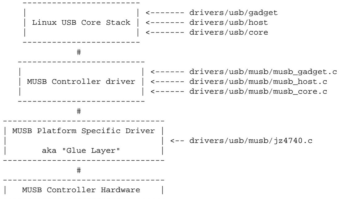
As outlined above, the glue layer is actually the platform specific code sitting in between the controller driver and the controller hardware.
