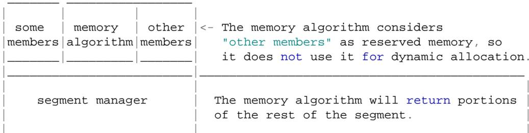
The **segment manager** initializes the memory algorithm and tells the memory manager that it should not use the memory where the rest of the **segment manager's** member are placed for dynamic allocations. The other members of the **segment manager** are a **recursive mutex** (defined by the memory algorithm's `mutex_family::recursive_mutex` typedef member), and **two indexes (maps)**: one to implement named allocations, and another one to implement "unique instance" allocations.
