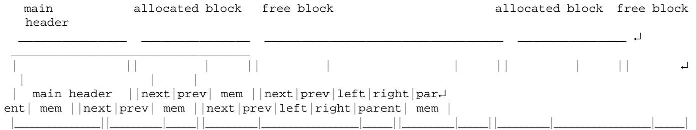
This allocation algorithm is pretty fast and scales well with big shared memory segments and big number of allocations. To form a block a minimum memory size is needed: the sum of the doubly linked list and the red-black tree control data. The size of a block is measured in multiples of the most restrictive alignment value.
